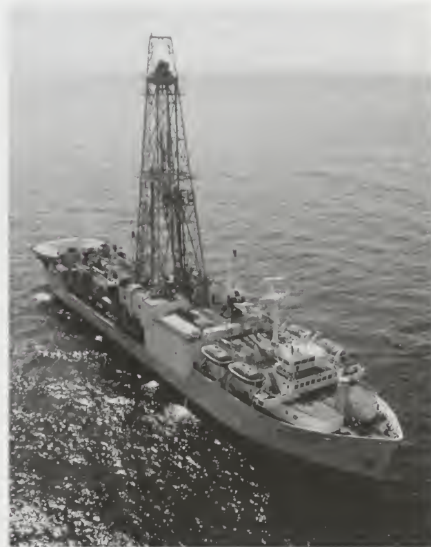
Figure 5: "JOIDES Resolution," a deep-sea drilling vessel that uses a computer-controlled, acoustic dynamic positioning system to maintain location over the drilling site. The derrick is visible amidships.
